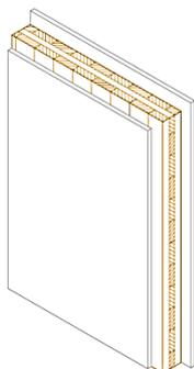
2.5 mm fire-protection plasterboard
