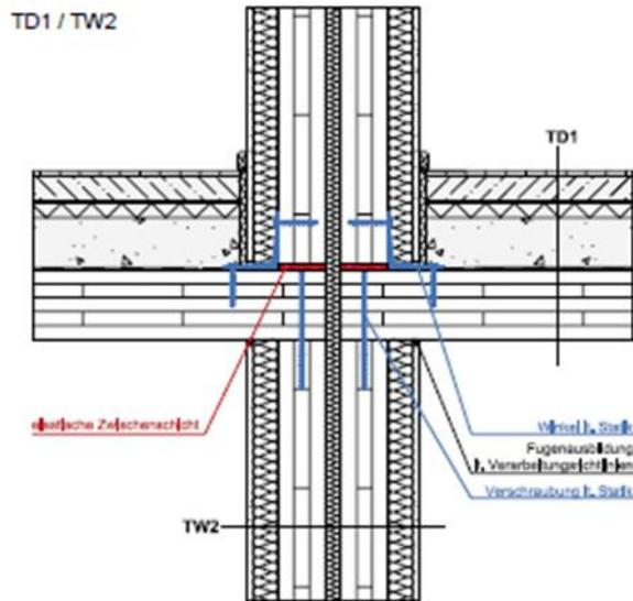
**Elastic bearings** are required **above the ceiling** in the case of cross-laminated timber ceilings with a timber soffit (without a suspended ceiling) and mechanically-isolated facing panels on the walls.
