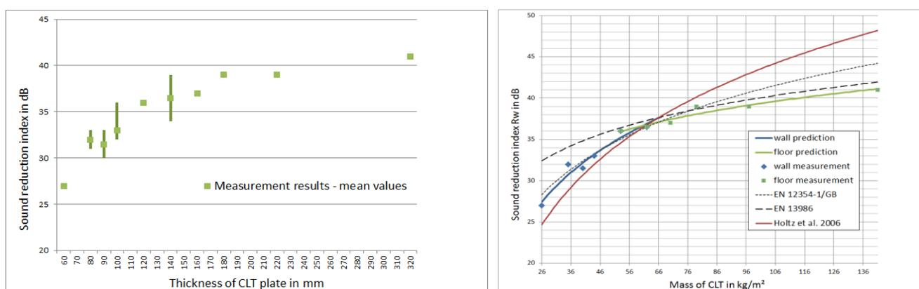
The left figure shows measurement results (mean values and variance) for airborne sound insulation of a CLT plate. The right figure shows the results graphically of the two equations in relation to the measurement results. Standardized equations and calculation model have also been calculated and are pictured as well.
