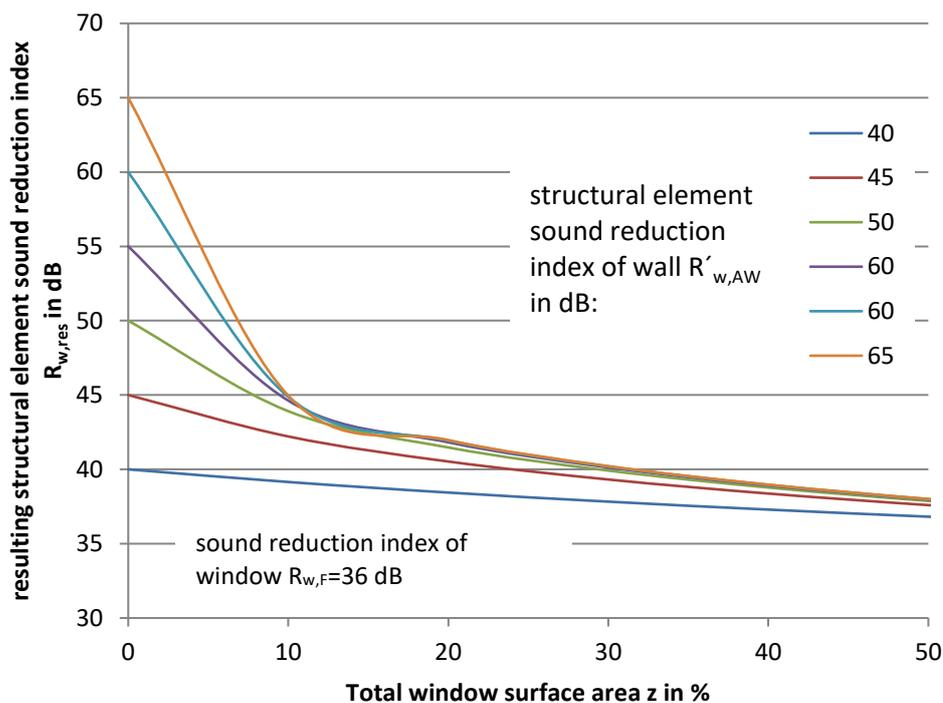
The diagram shows the  $R'_{res,w}$  depending on the window surface area when installing a window with  $R_{w,F} = 36$  dB.
