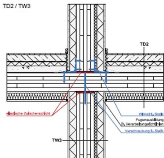
**Mechanically-isolated facing panels, suspended ceilings and elastic bearings above and below the ceiling** are always required on continuous ceilings above different parts of the building.
