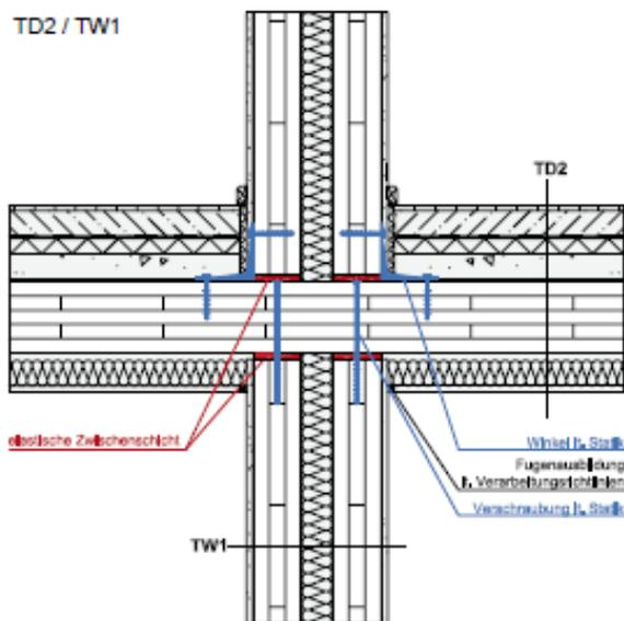
**Elastic bearings** are required **above and below the ceiling** in the case of suspended ceilings without mechanically-isolated facing panels on the walls.
