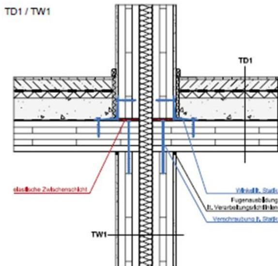
**Elastic bearings** are required **above the ceiling** in the case of cross-laminated timber ceilings with a timber soffit (without a suspended ceiling) and without mechanically-isolated facing panels on the walls.
